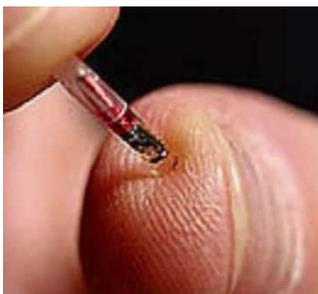
set up to emulate an EM41xx style chip, which is a very common low frequency chip type. In this mode, it works with common EM41xx based readers available through many hobby electronics shops and electronics outlets. The xEM can also emulate HID **ProxMark II** card IDs, which are commonly used in corporate access control applications. Several commercial or "off the shelf" systems are
