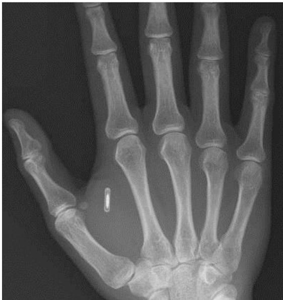
frequency 13.56MHz transponder based on the ICODE SLI chip. This chip type is ISO15693 compliant but is not NFC compliant. The xIC has 128 bytes of user programmable memory but has no security features. The xIC is supported only on some NFC devices which contain a reader chip from NXP. While the xIC will work with any ISO15693 proximity reader, it cannot be expected to work reliably with all NFC devices. We supply the xIC for people who have a specific need for this particular chip type.]
